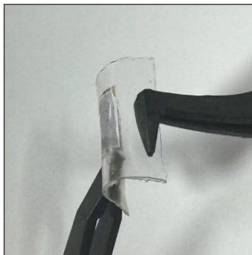
Fig. S15 Picture of a fabricated flexible PUF chip on a PDMS substrate.
